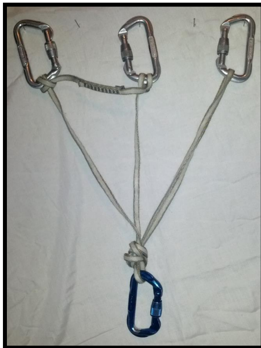
Three leg, two anchors clove hitched, loop on third anchor, tied master-point
