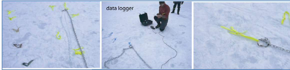
Figure 9 (left) shows multiple Abalakov slow pull testing in action; (middle) logging data and quickly moving the pull testing device from anchor to anchor; (right) showing the strongest Abalakov configuration and material used (1" tubular webbing).
