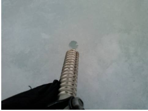
Figure 1 Placing a screw into an existing hole is called re-boring.
