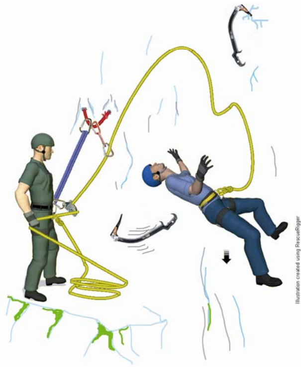
Figure 17 Multi-pitch scenario: Leader falling onto a single ice anchor (in this case a single horizontal Abalakov) that the belayer is also attached to in the UIAA fall test scenario, a potentially deadly combination.
