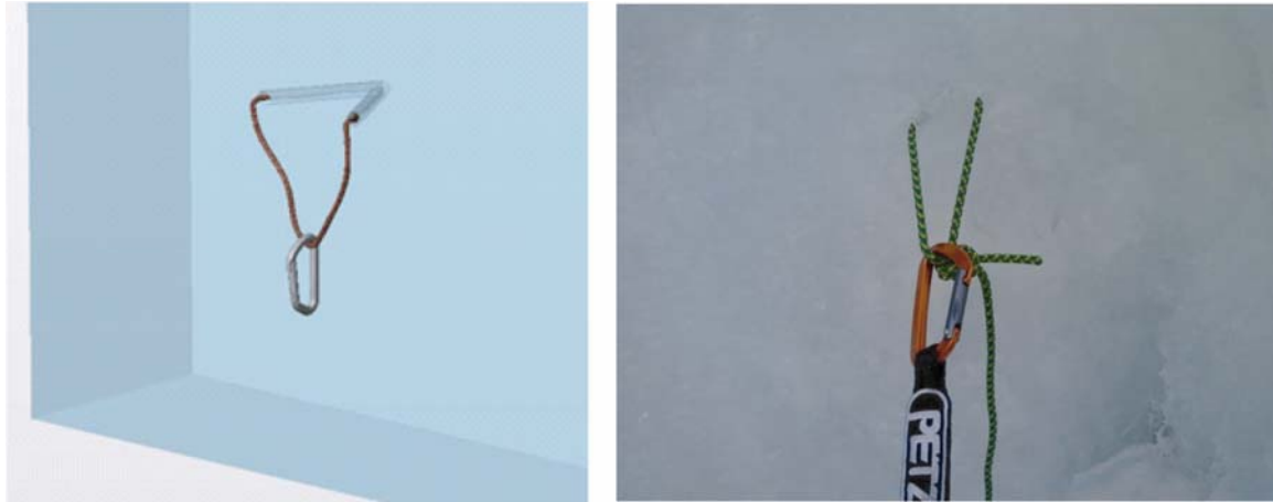
Figure 2 shows a traditional horizontally made Abalakov ice anchor. Notice that in the example on the right, the cord is tied off with a flat overhand. This is usually acceptable for rappelling only and not advocated for lead configuration.
