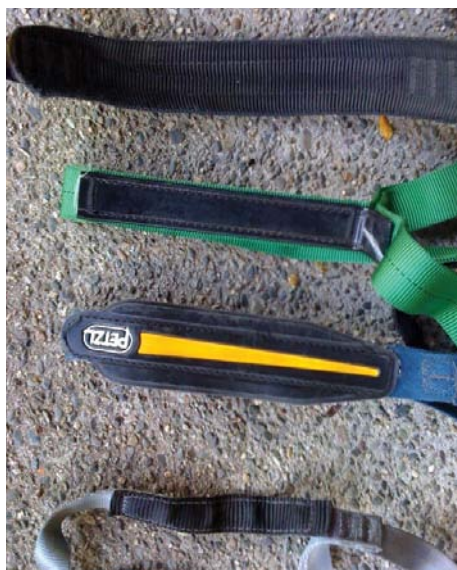
Showing aider step width. From top to bottom: Yates Aid Ladder, Metolius Aider, Petzl WallStep, Petzl GradiStep.
